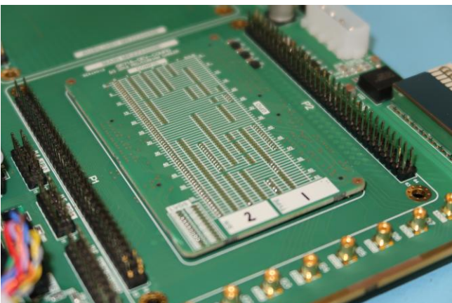
Figure 4-7: Installed Interface Configuration Board
